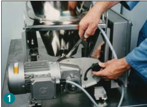
1 All components are accessible from the rear of the feeder instead of the discharge side. Simply loosen the bolt and the hand knob on the back of the coupling bell.
