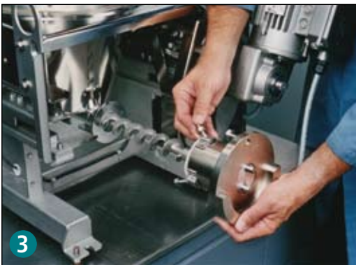
3 For easy removal of the helix, loosen the nuts of the three screws on the back of the coupling bell, allowing for fast helix style, and diameter changes.
