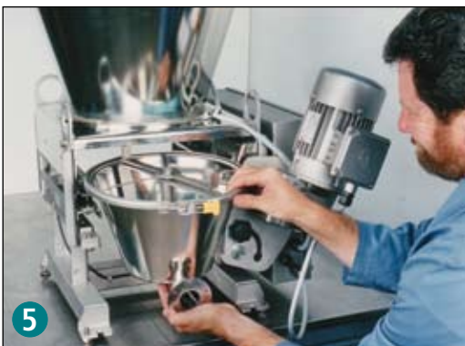
5 The feed hopper slides out for cleaning, replacement or maintenance.
