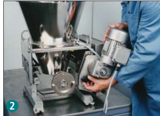
2 Swivel motor and drive assembly back and tighten hand knob for complete access to all internal components for easy cleaning, reconfiguration, and maintenance.
