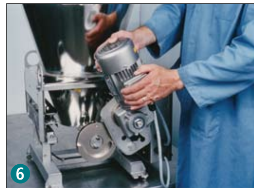
6 Replace feed hopper, reposition motor and drive assembly, tighten hand knob and bolt, and you're ready to run – all in under two minutes.
