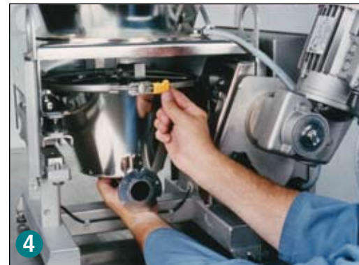
4 Release band clamp and lower the feed hopper to disengage the agitation system.
